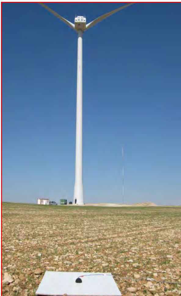
Sound power level measurement according to standard IEC 61400 part 11
