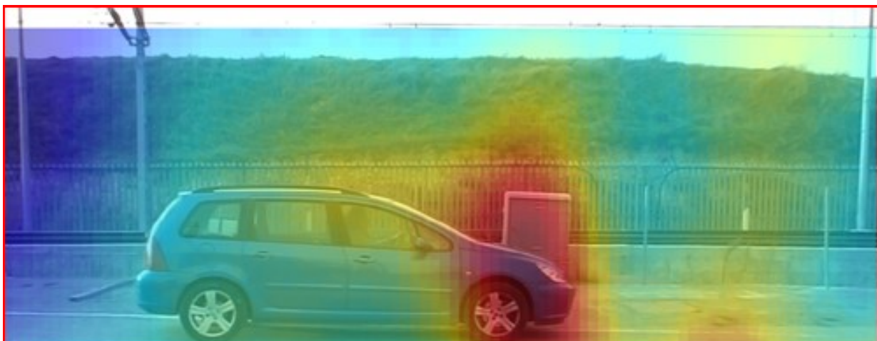
Noise sources localisation on a movement car
