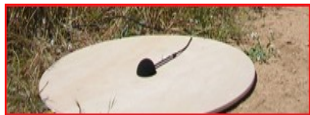
Sound power measurement according to IEC 61400 part 11
